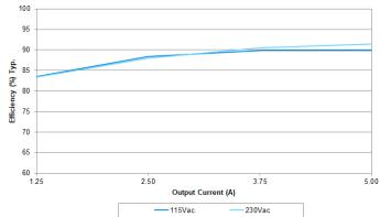
Fig. 2 Efficiency VS Output Load at 24V
