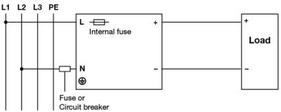
Fig. 15 2 of 3 Phase System Input Operation Connection Diagram
