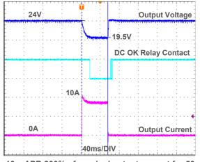
Fig. 10 APB 200% of nominal output current for 50ms
