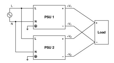
Fig. 12 Parallel Operation Connection Diagram
