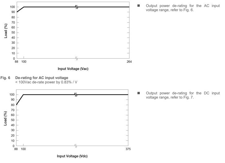
Fig. 7 De-rating for DC input voltage < 100Vdc de-rate power by 1.67% / V
