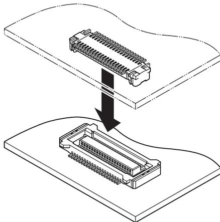
0.4mm pitch, SMT, low profile connector with parallel connection.
