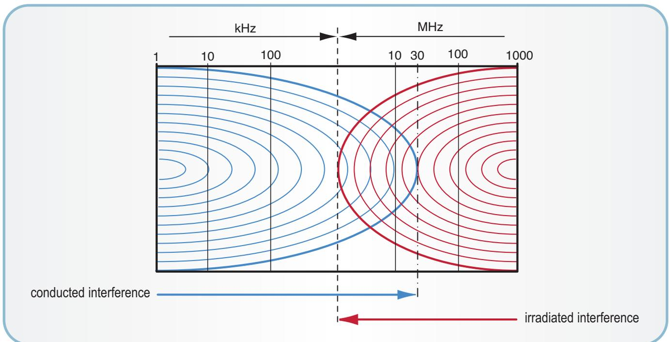
By test convention, **interference with frequency up to 30 MHz** is considered to be conducted and **irradiated with frequency above 30 MHz up to 1 GHz**.
