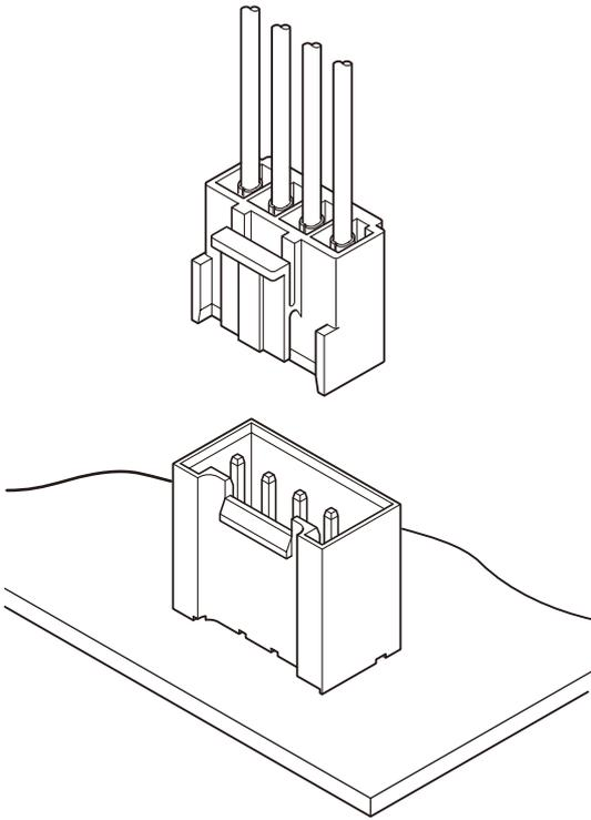
**Header for 3.96mm pitch VH connector for use specifically with resin coated ("potted") PC boards.**
