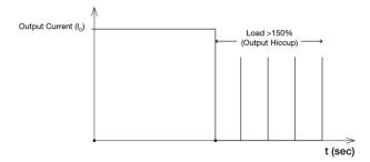
It is not recommended to prolong the duration of  $I_{\rm O}$  when it is <150% but >100%, since it may cause damage to the PSU.
