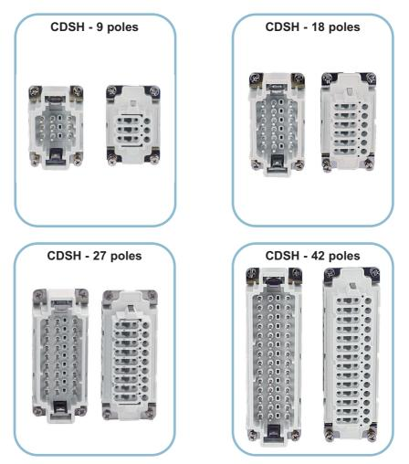
Each of the spring terminals has an actuator button, suitably shaped and incorporated in the cavity. When this button is pressed, it triggers the closure of the spring device of the corresponding terminal, safely and reliably connecting the conductor to its respective electric contact in the connector.
