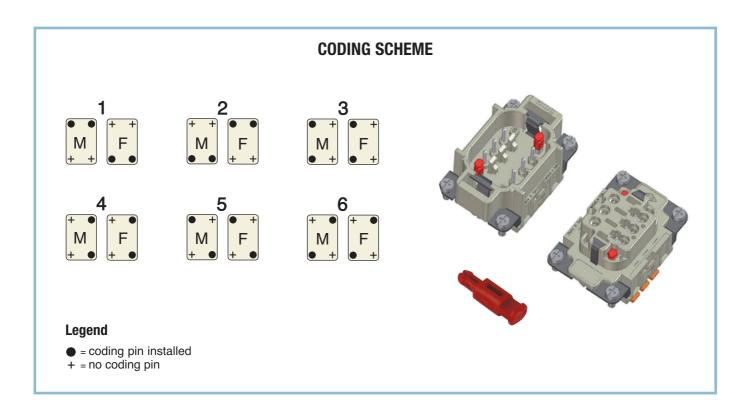
The CR CDS coding pins can also be used in combination with other CR 20 / CRM / CRF / CR 72 metal pins instead of insert fixing screws in order to increase the number of possible combinations.
