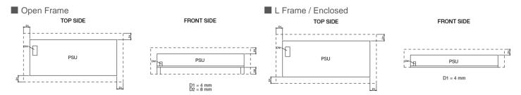
For safety reasons, please ensure the mounted device is kept at ≥ 4mm (0.16 inch) safety distance at all sides from other components and equipments. Please insert an insulation sheet between the system and product, if the safety distance is less than 4mm (0.16 inch).
