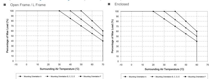
Fig.1.1 De-rating for Mounting Orientation A
