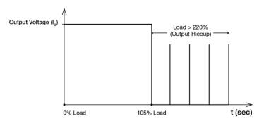
It is not recommended to prolong the duration of  $I_0$  when it is <220% but >100%, since it may cause damage to the PSU.
