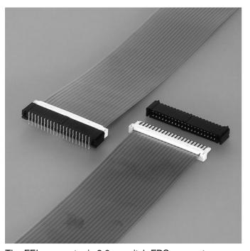
The FEL connector is 2.0mm pitch FPC connector suitable for environments in automotive compartment. The FEL connector is different from the conventional ZIF type connector, reliable connection is greatly improved by using a general housing lock for an automotive connector.
