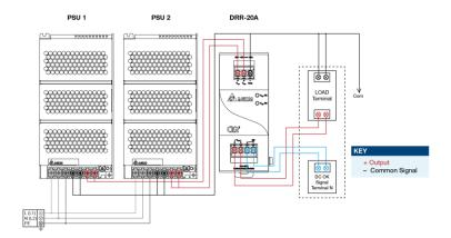
Fig. 3 Redundancy Operation Connection Diagram
