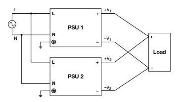
Fig. 4 Parallel Operation Connection Diagram
