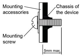
Only use M3 screw ≤ 5mm (0.19 inch) through the base mounting holes. This is to keep a safety distance between the screw and internal components.
