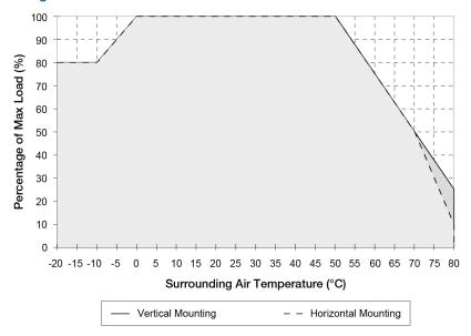
Fig. 1 De-rating for Vertical Mounting Orientation
