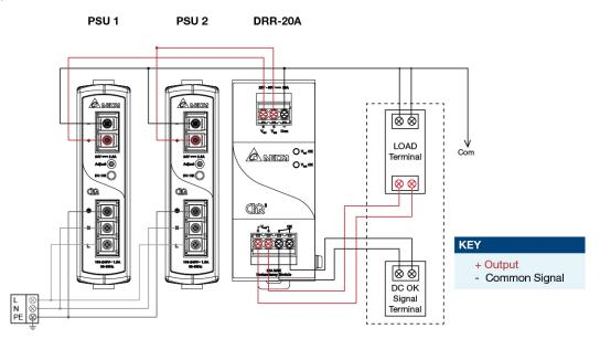
Fig. 3 Redundancy / Parallel Operation Connection Diagram
