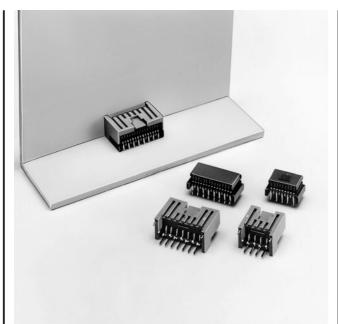
Self-supporting style board to board connectors. Both plugs and receptacles are supplied radial-tape mounted (conforming to JIS C 0805 tape specification), which can be mounted by versatile, radial component pick and place machines. Automatic mounting is possible up to 15 circuits.
