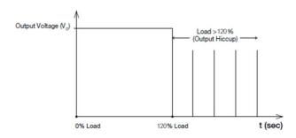
Additionally, if the  $I_0$  is < 120% but > 100% for a prolong period of time (depending on the load), the Over Temperature Protection (OTP) will be activated due to high temperature on critical components. The power supply will then go into "Hiccup mode" until power supply cool down.
