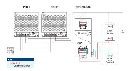
Fig. 3 Redundancy / Parallel Operation Connection Diagram
