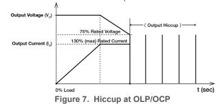
Additionally, if the lout is >100% for a prolong period of time (depending on the load), the Over Temperature Protection (OTP) may be activated due to high temperature on critical components. The power supply will then go into latch mode.
