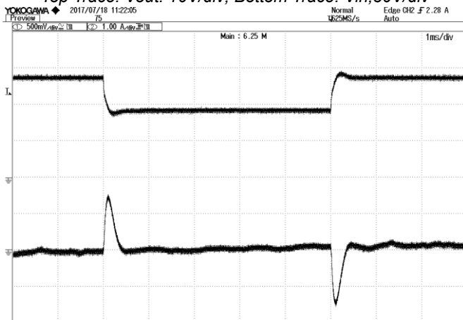
Figure 3: Turn-on transient at full load current (10ms/div). Top Trace: Vout: 10V/div; Bottom Trace: Vin, 30V/div
