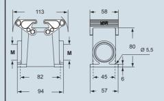
The surface mounting, high construction housings are supplied with an open threaded entry and diametrically opposite a closed threaded entry which can be opened by the user if required (with suitable tool).
