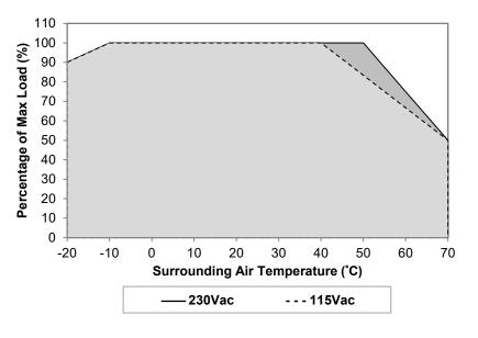
Fig. 1 De-rating for Vertical Mounting Orientation -10°C to -20°C de-rate power by 1% / °C > 40°C de-rate power by 1.67% / °C @ 115Vac > 50°C de-rate power by 2.5% / °C @ 230Vac
