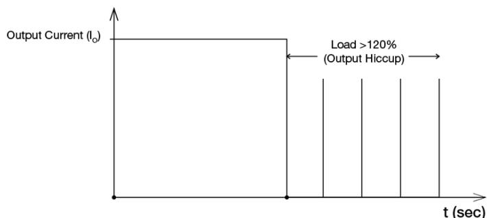
It is not recommended to prolong the duration of  $I_o$  when it is <120% but >100%, since it may cause damage to the PSU.
