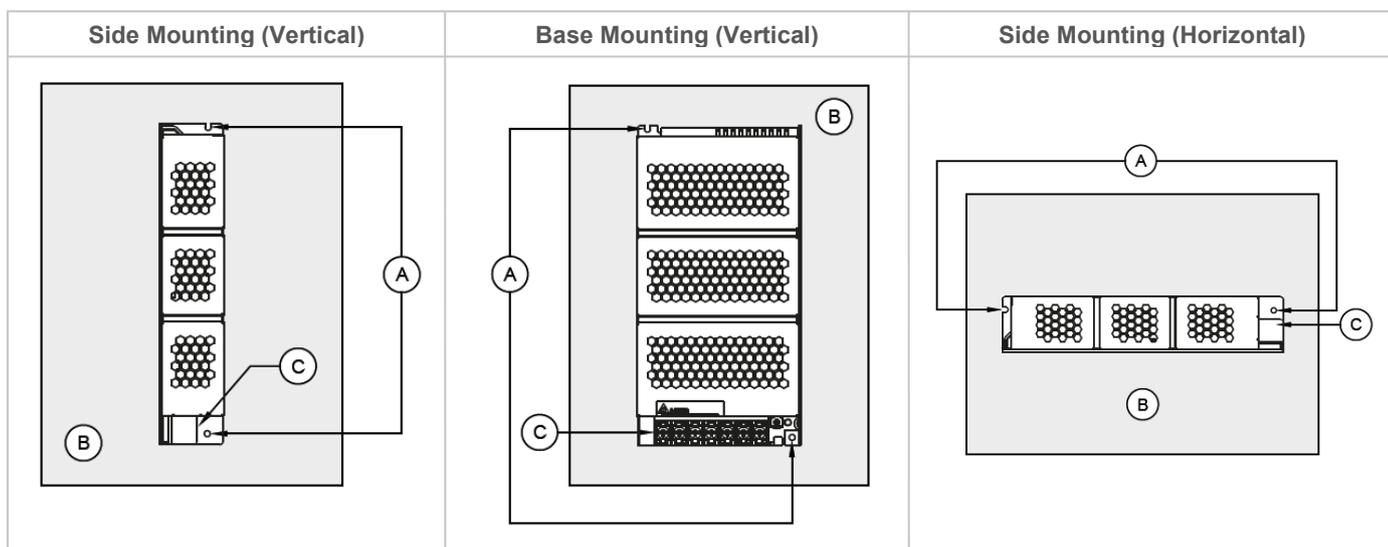
Fig. 2 Mounting Orientation
